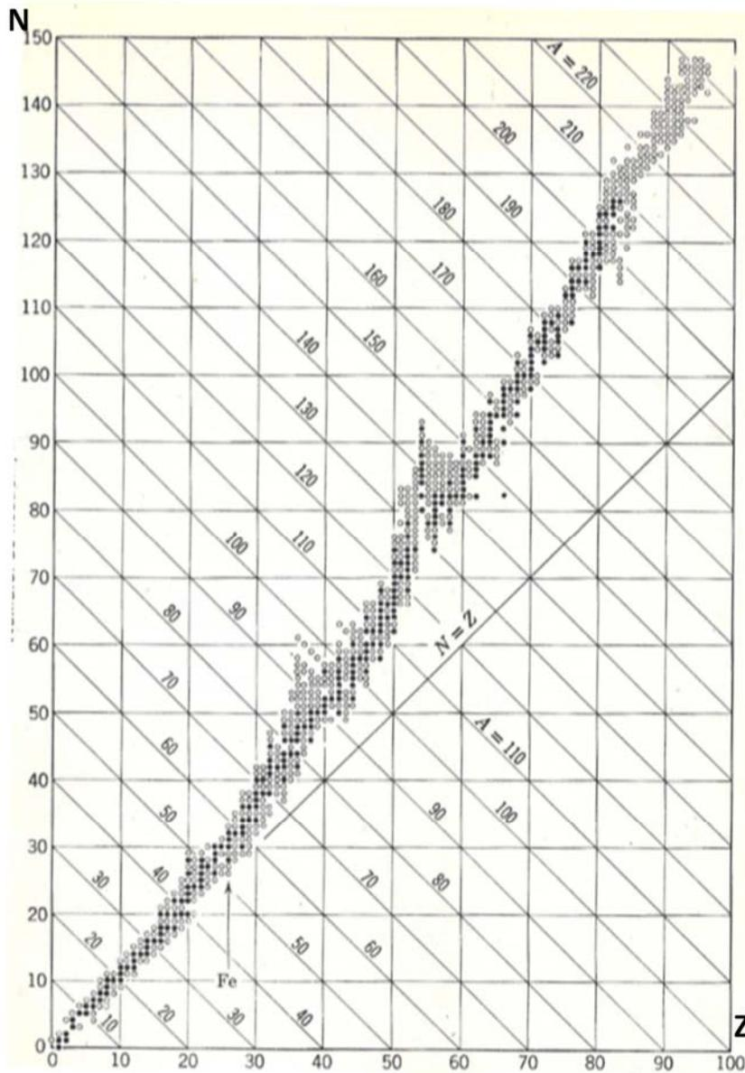
Fig. 1. Diagram of atomic cores (atomic nuclei)
