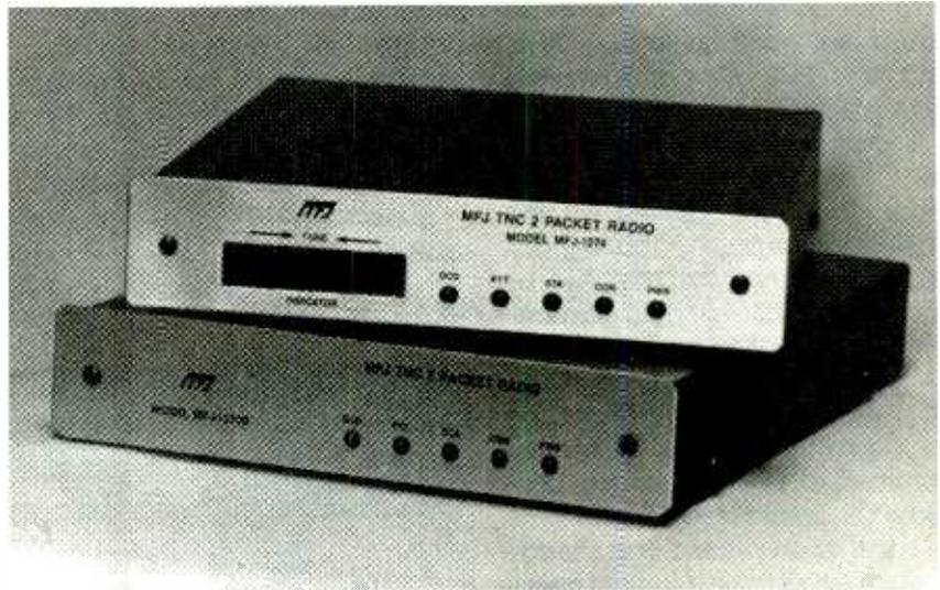
*MFJ offers TNCs for HF and VHF packet radio, several of which are based on classic TAPR designs. Thousands of units similar to this rugged basic model are used as digipeaters, nodes, and BBSs, and in commercial applications.*
