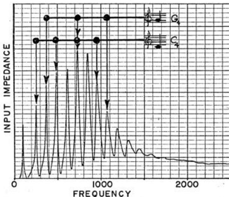
Figure 7: Impedance of a modern B-flat trumpet
