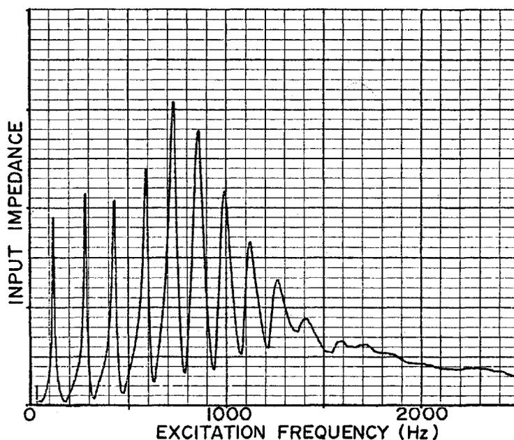
Figure 6: Measured impedance curve for a complete cornet
