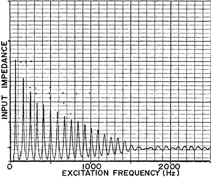
Figure 5b: Impedance modified by adding a bell
