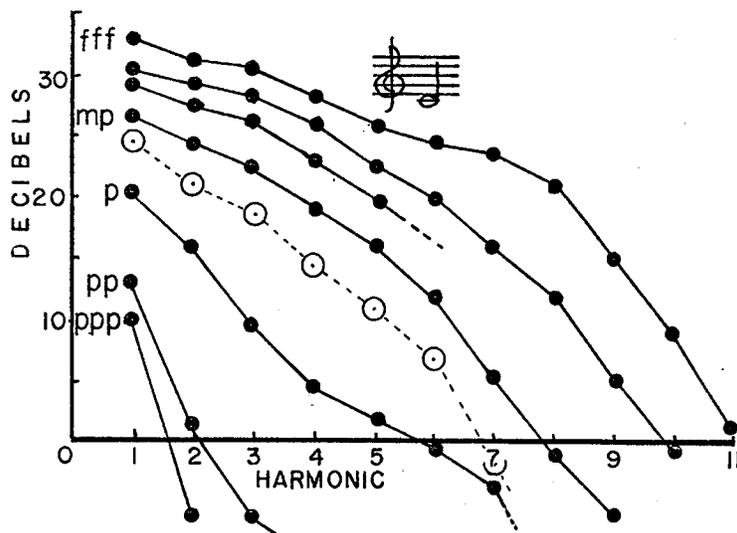
Figure 13a: Internal partials of the written  $C_4$  (concert B-flat<sub>3</sub>) on a modern trumpet
