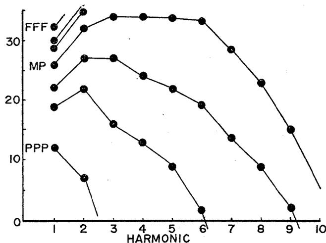
Figure 17a: External spectra of written  $C_4$  (concert B-flat<sub>3</sub>) on a modern B-flat trumpet
