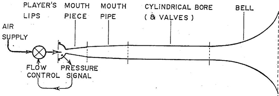
Figure 1: Basic structure of a brass instrument
