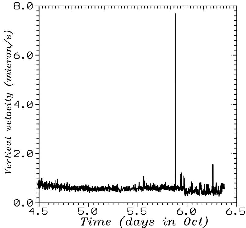
Figure 14: Maximum ground velocity in Aurora mine.
