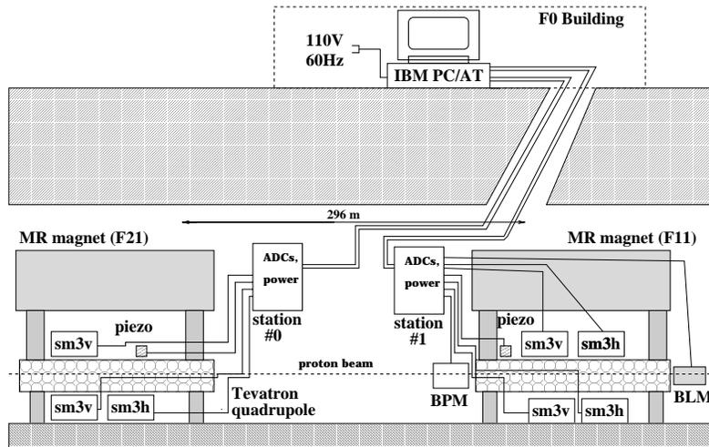
Figure 2: Scheme of measurements in the Main Ring tunnel.
