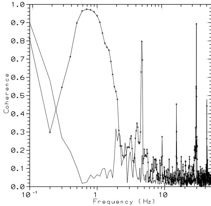
Figure 13: Coherence between signals of the vertical Tevatron beam orbit motion and the F11 magnet vibrations (marked line) and between the orbit and the tunnel floor.
