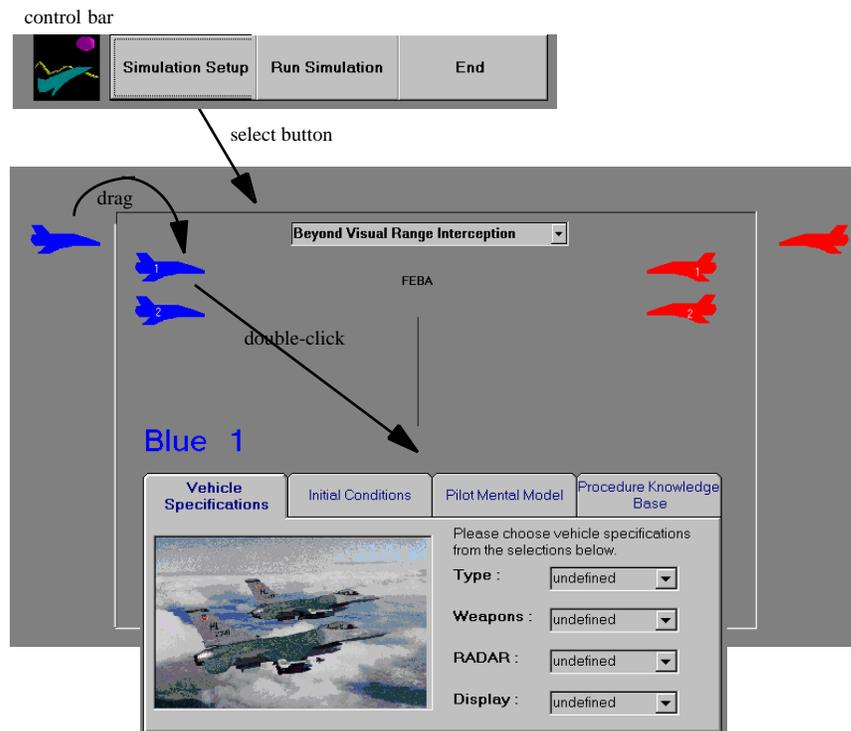
Figure 2.3-1: Aircraft Configuration Using the Simulation Setup Navigator
