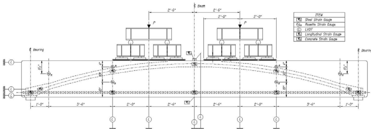
**Figure 5. Elevation of Test Set-Up and Instrumentation Plan**
