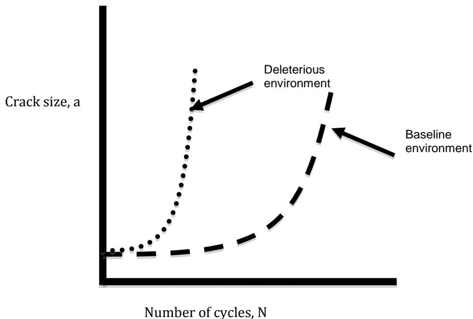
**Figure 9-5: Diagram Depicting the Potential Effect of a Deleterious Chemical Environment on Fatigue Crack Propagation (the amount of the effect(s) is dependent on numerous parameters mentioned in Figure 9-4).**
