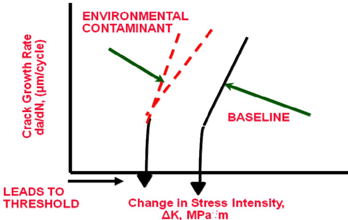
**Figure 9-6: A Depiction of Fatigue Crack Propagation Data Plotted on  $da/dN$  versus  $\Delta K$  Axes**
