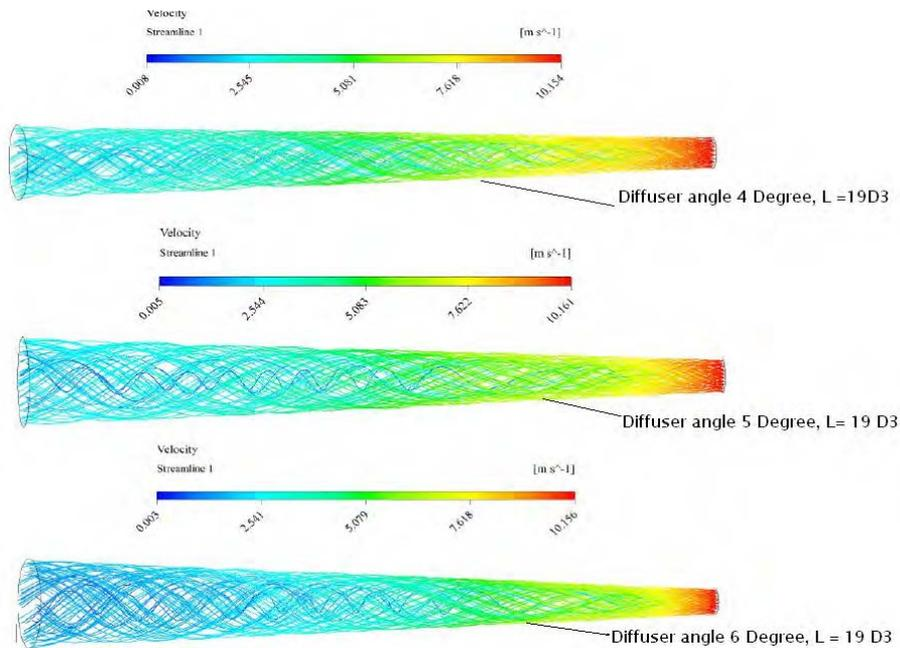
Figure 7. Velocity stream lines for different diffuser angle at constant length  $19D_3$
