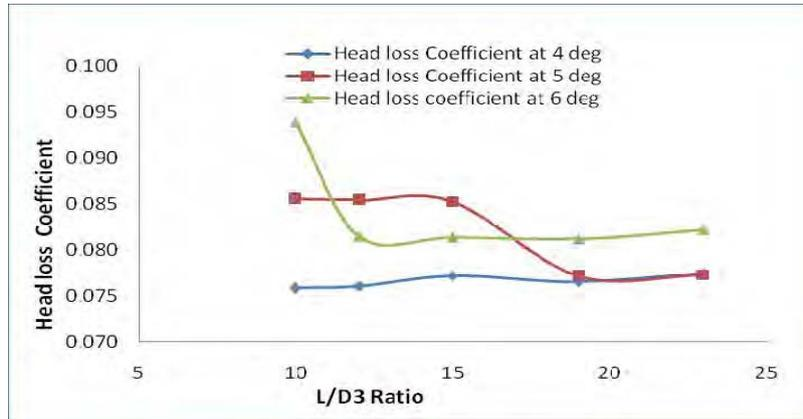
Figure 4. Head loss variation with length at different diffuser angle
