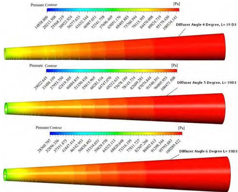
Figure 8. Pressure contours for different diffuser angle at constant length 19D<sub>3</sub>
