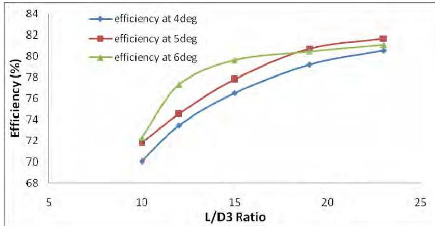
Figure 6. Variation of efficiency at different  $L/D_3$  ratio and diffuser angle
