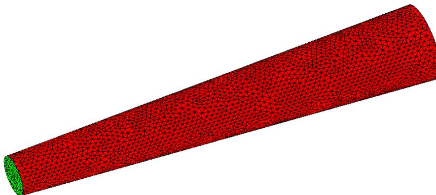
Figure 3. Meshing of the draft tube
