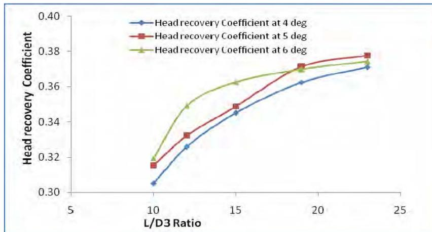
Figure 5. Head recovery with  $L/D_3$  ratio at different diffuser angle
