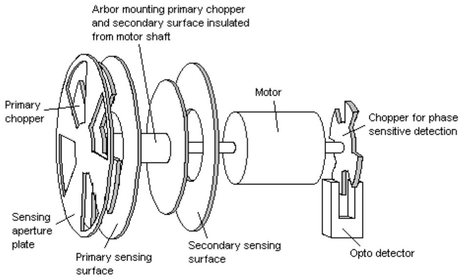
**Figure 1: Basic arrangement for 'back to back' fieldmeter**
