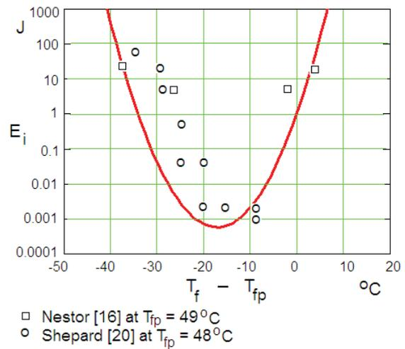
Fig. 13. Comparison of eqn (5) with test data for variation of the MIE with the temperature  $T_f - T_{fp}$  of JET A fuel at  $h_a = 4270$  m (14 000 ft) altitude. Experimental data from J. Nestor [16] and J.E. Shepard [7, 20].
