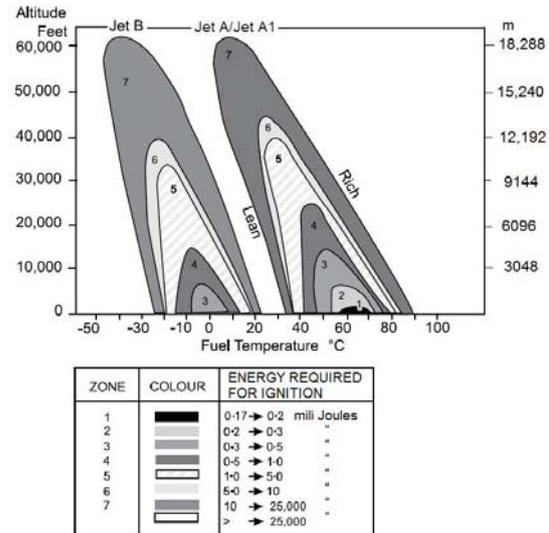
Fig. 9. Flammability envelopes and estimated minimum electrical ignition energies for Jet A/Jet A-1 and Jet B fuels. Source: British Aerospace [7].
