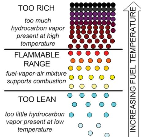
Fig. 8. Flammability concept for fuel vapor-air mixture [13].
