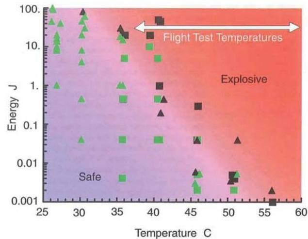
Fig. 15. MIE  $E_i$  versus fuel temperature  $T_f$  at pressure of 0.585 atm to ignite a sample of Jet A fuel-air mixture according to J.E. Shepard [21]. The green data points represent samples that did not ignite, the black points exploded. The squares are test simulating 0.189 m<sup>3</sup> (50 gallon) of fuel and the triangles represent a quarter-fuel tank.
