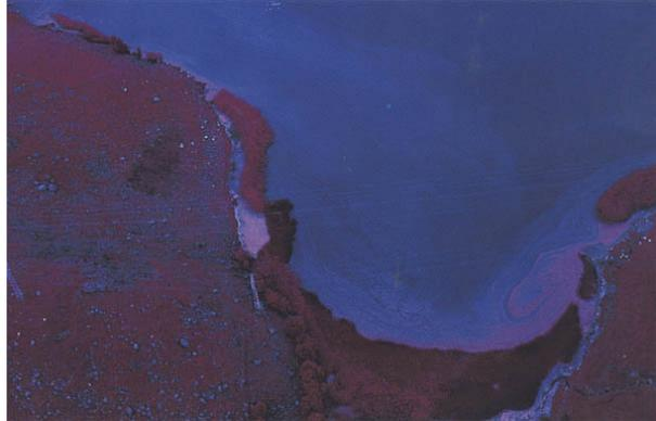
**Figure 2.2G** Use of a barrier or boom to keep surface scums of algae and cyanobacteria away from water offtake structures (Photograph courtesy of Peter Baker, Australian Water Quality Centre)
