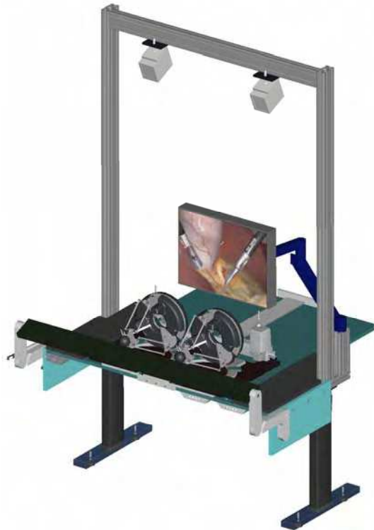
Figure 12. CAD depiction of the proprietary developed telesurgical workstation (master console)
