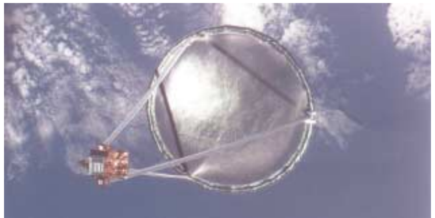
Right: The 14-meter Spartan 207/Inflatable Antenna Experiment in flight.
