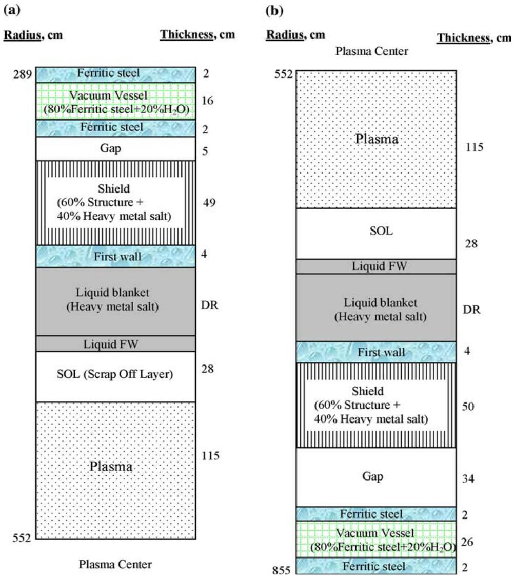
Figure 1. One-dimensional APEX model (a) inboard, (b) outboard [2].
