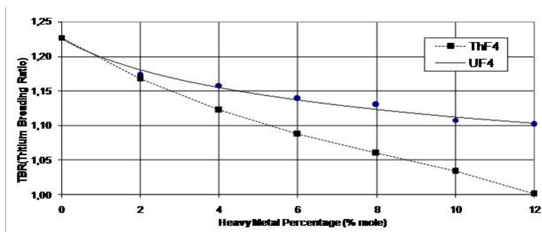
**Figure 3.** The variation of TBR values versus the heavy metal fraction in the liquid medium.
