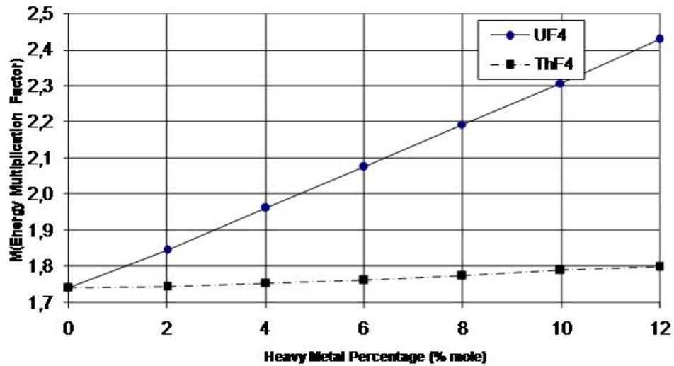
**Figure 4.** The variation of M with the heavy metal fraction in the liquid medium.
