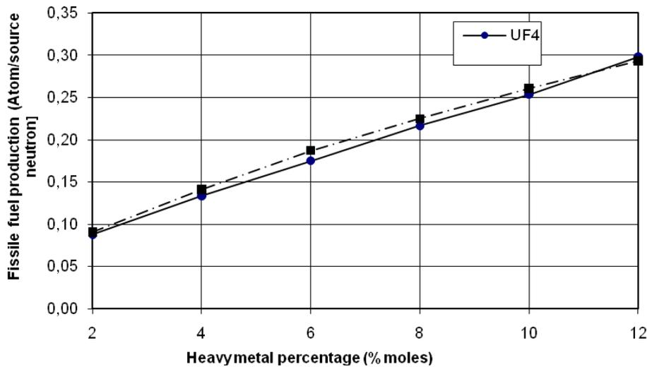
**Figure 5.** Fissile fuel production in the liquid wall versus the heavy metal percentage.
