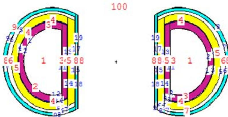
Figure 2. Cross-sectional view of APEX fusion reactor model designed in MCNP-4B [6].
