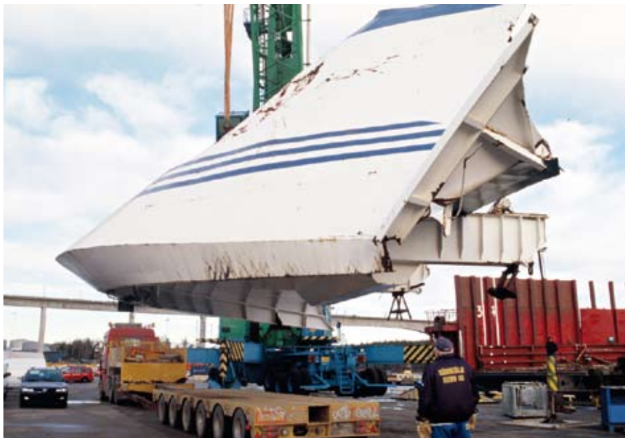
Fig. 2. The bow visor from M/S Estonia. Photo: Gunnel Ilonen, the Maritime Museum.
